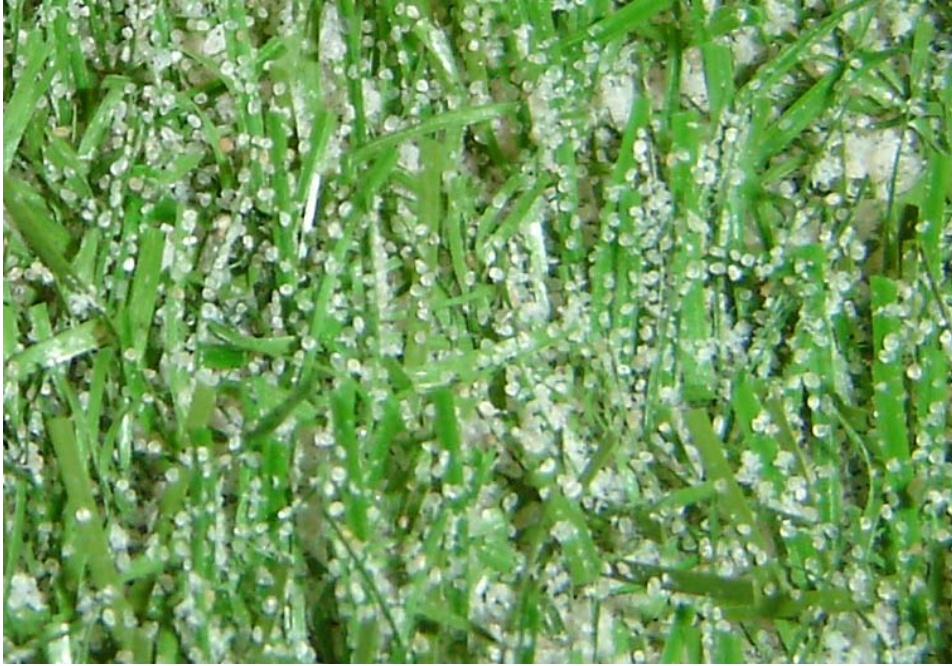
Photograph of carpet after 20,000 cycles simulated wear. Flexsand sticking to pile due to static electricity; damping sample prevents this phenomenon from occurring.
