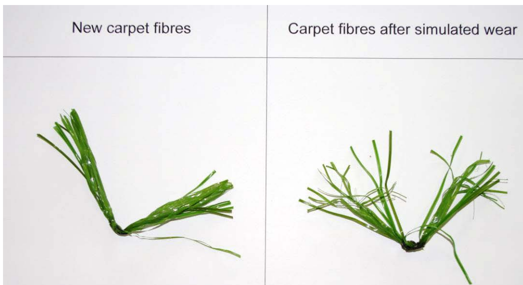
Photograph of fibres before and after 20,000 cycles simulated wear
